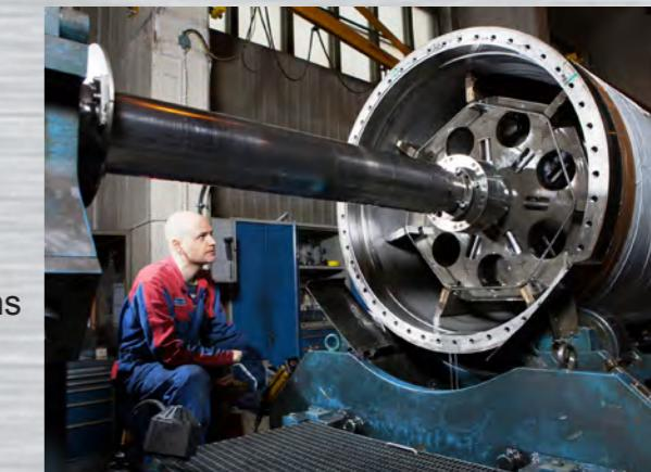
**Internal turning:** Ø 1500 mm x 10500 mm up to 60 tons
